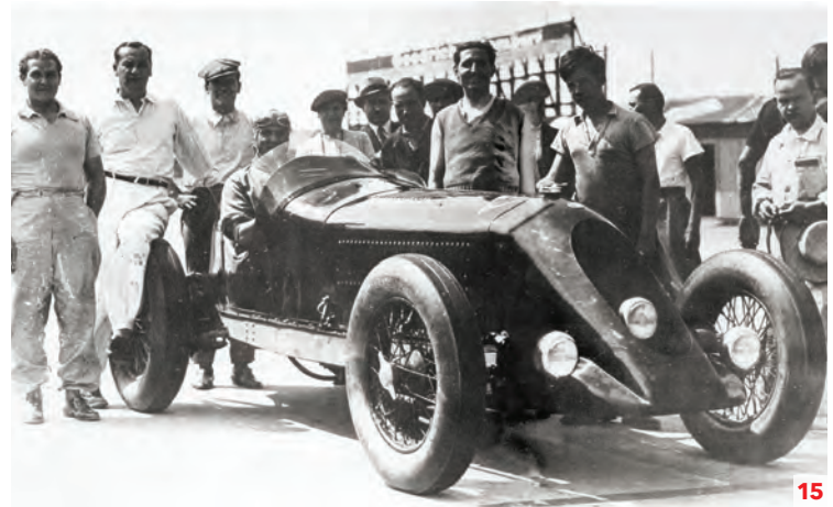
15 In 1935, Chinetti staged two record attempts at Montlhéry using 8C chassis 2211135. Figoni constructed an aerodynamic radiator cowl with no grille. The radiator remained in place and the cowl acted as an extension, much like the one Figoni had created for 2111018 in 1932. The front brakes were dismantled, and three driving lamps fitted. In this group photo taken prior to the start of the first record-breaking attempt on 7th August, 1935, Chinetti is at the wheel. The body was dark as it had been repainted by Figoni, while the light chassis rail reflected the previous colour of 2311235. Note the quadrifoglio on the bonnet and the Maserati filler cap on the radiator. Both record attempts failed (Collection Serge Pozzoli)
