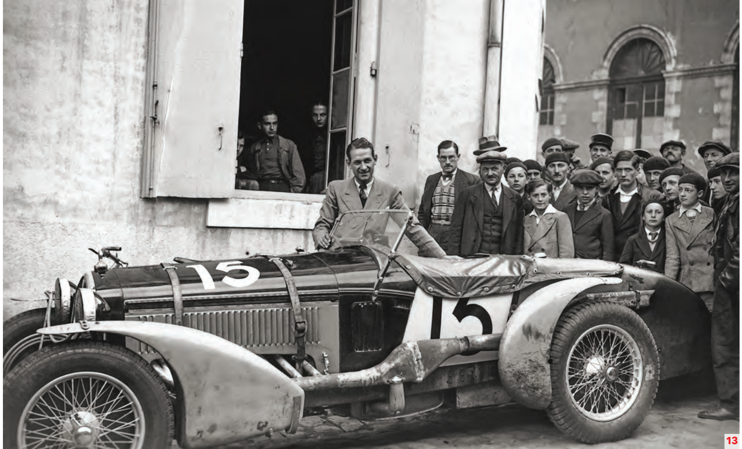
13 Raymond Sommer presenting 8C chassis 2311212, his 1935 Le Mans car, for press and fans. The diagonal cut where the Touring beltline stops clearly demonstrates where Sommer's now well-used Zapon-covered Weymann-type Figoni body was mounted on his donor car; 1935 was the last time this coachwork and its accessories ran at Le Mans (Collection Flavien Marçais)
